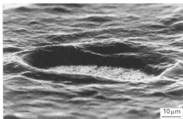
Figure 6 Scanning electron micrograph of an amorphous carbon film with a pin-hole in which silicon nitride can still be seen.
